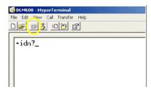
The supply model information ID string, similar to the example shown below, should appear indicating the supply communication is operational.
