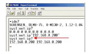
NOTE: assigning a new IP address using this method, forces the Ethernet communication into using a "Static IP Address" and power to the supply's power switch must be cycled in order for the change to take effect.
